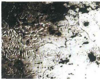
图3 四川绵阳西汉铁铲 1930 网状浮凸组织较多 X100 Fig.3 Reuecular ghosting structure in iron shovel 1930 unearthed from Mianyang, Sichuan (the Han Dynasty) X100 (etchant: 4% Nitah)
